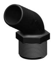
TruDesign Tails are moulded from a glass reinforced nylon composite. High strength, high-modulus glass fibres impregnated into the nylon provides dramatic strength, stiffness, toughness, and dimensional stability. TruDesign Tails eliminate the corrosion and electrical bonding problems associated with metallic fittings. The Tails are designed for twin hose clamps, and to not crush under high load conditions.
